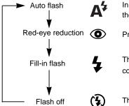
In low light conditions, flash will automatically fire to obtain the correct exposure.
